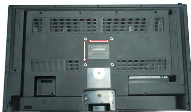
Mounting Specification : **100mm x 100mm** using screw size **M6**. Length of screw should not exceed **8mm**. Please Note : The **8mm** length of screw refers to how deep the screw can go inside the mounting holes. When you're buying screws, you should add the original 8mm to the thickness of your mounting plate in order to get the total screw length.
